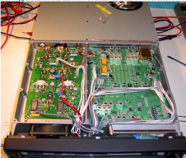
5. Now remove 6 golden screws of receiver board. Do not pinch the cables which hide the screws.
